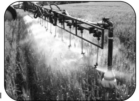
Figure 5 - Turbo FloodJet – alternating forward and backward nozzle set up for fungicide application for FHB suppression.
